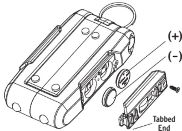
**1.** The batteries for the flashlight are under the On/Off switch. Using a small Phillips screwdriver, turn counterclockwise to remove the screw. Gently lift the Switch Assembly up and out to expose the Battery Compartment.
