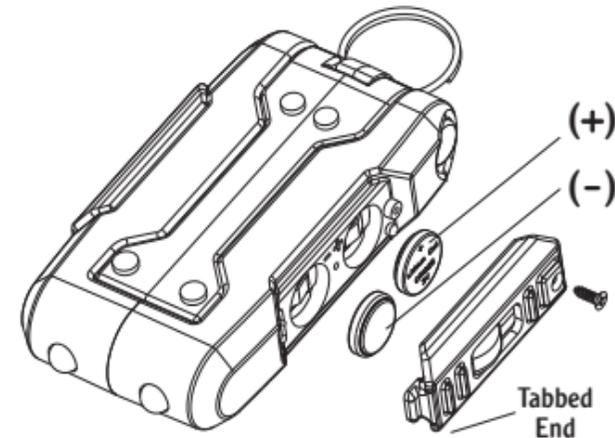
1. The batteries for the flashlight and work lights are under their On/Off switches. Using a small Phillips screwdriver, turn counterclockwise to remove the screw next to the switch that needs new batteries. Gently lift the Switch Assembly up and out to expose the Battery Compartment.
