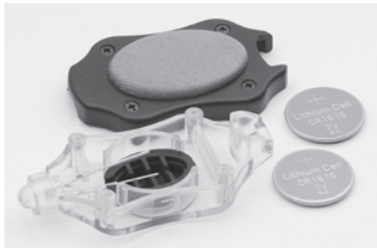
Two CR1616 Batteries Positive Side (+) Up
