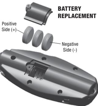
1. Loosen screw, remove batteries (captive screw remains in housing).
