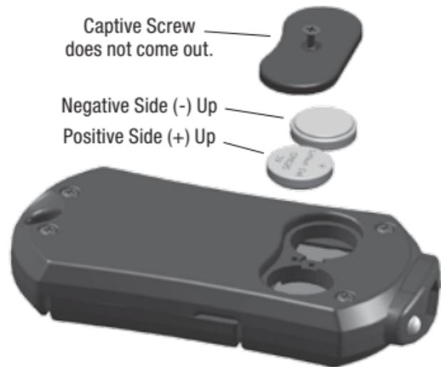
1. Loosen screw, remove batteries (captive screw remains in housing).
